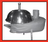
Shand & Jurs insulation jackets provide heat retention for equipment in cold weather environments. Construction of the insulating jacket is silicone impregnated woven glass cloth lining with 1'' thick fiber glass material. The jacket is easy to install and remove in the field.
