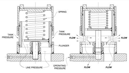
To open the valve, hydraulic fluid pressure is applied to the plunger which moves to open the normally closed piston.
