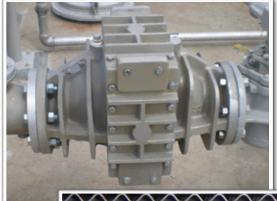
The Shand & Jurs 94309 Flame Arrester (Plate Element) quenches a flame front by cooling the flame to below the ignition temperature. As the flame front enters the arrester, it is intercepted by the arrester element specifically designed to provide a precise path for the flame to follow.
